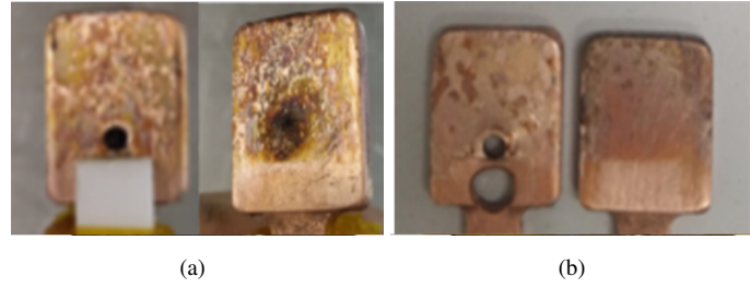
Figure 3.8: Deposition and erosion on the discharge channel surfaces after repetitive firing. Example featuring h=0.5 cm (a) and 1.5 cm (b), l = 1.5 cm, V_0 = 1000 V, C = 5 \mu\text{F} with Battery 1 (1) after 200 firings.
