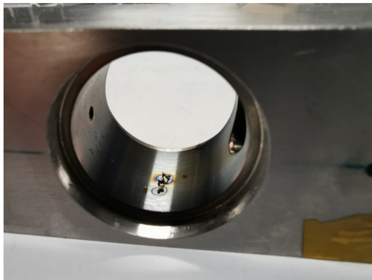
Figure 6.5: Photography of the central connector of the IC after the campaign.
