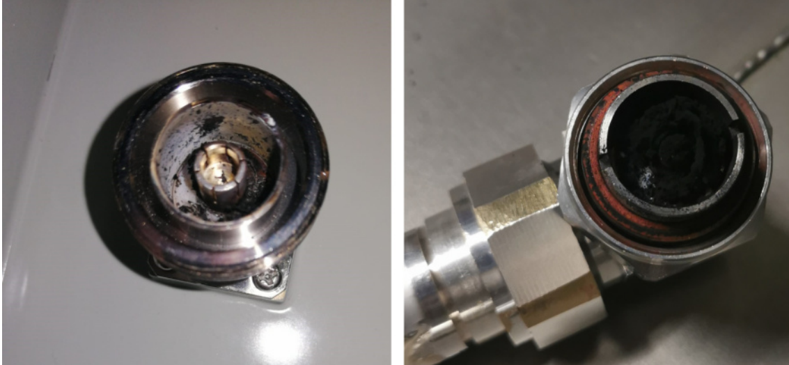
Figure 6.3: 7-16 DIN coaxial connector of the C2W 1 (left) and connector of the CC1 (right) after the experience.
