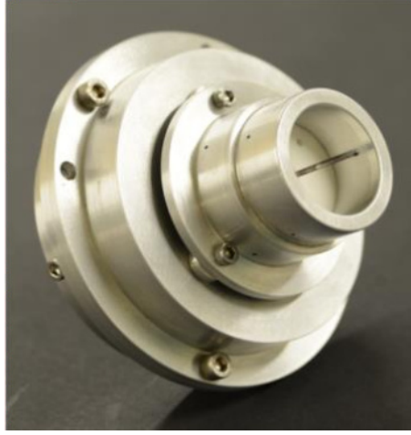
Figure 1.6: Picture of a 30 W ECRA thruster[44].
