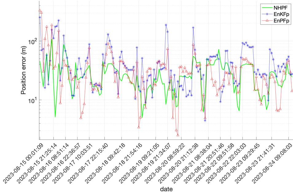
Figure 4.19: RMSEs in position for the three proposed algorithms which estimate the given \sigma_w . The solid blue line shows the EnKFup errors, the red line shows the EnPFup errors, and the green line shows the NHPF errors.
