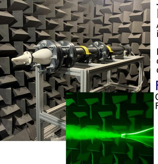
Jet Testing Facility Anechoic chamber to isolate jet noise effects
