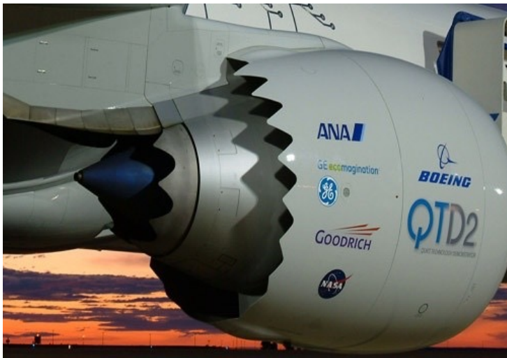
Boeing 787 Chevron Nozzle. Image extracted from Capt. Samarth Singh Wadalia LinkedIn.
